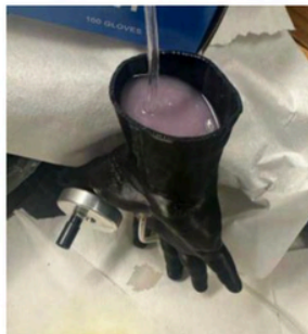
Casting of the silicon hand/wrist.
