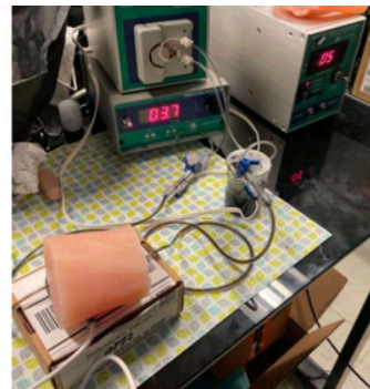
Phantom attached to pulse flow system.
