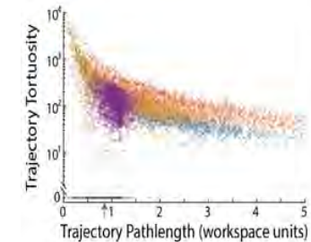
Figure 2: Trajectory pathlength versus trajectory tortuosity (integrated instantaneous curvature change normalized by pathlength) shows DDS subjects executed shorter and spatially simpler trajectories than other groups. The occasional sharp turns in DDS trajectories generated tortuosity similar to the smooth and simple arcs of vKF trajectories, although they’re typically shorter. ReFIT trajectories contained the most erratic changes in direction.
