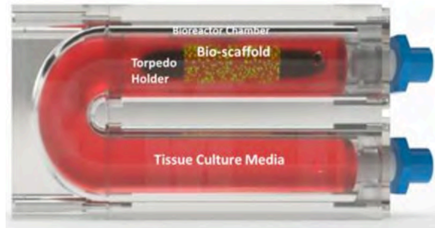
Figure: U-shaped bioreactor chamber used for dynamic-flow conditioning of MSC cells.
