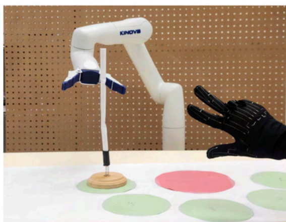
Fig 1. Photo of the experiment setup. The 6 DOF robotic arm (left) is being piloted by the participant (right) wearing a CyberGlove.
