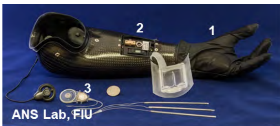
Fully assembled ANS-NEPH system and implant. 1) Instrumented Prosthetic Hand (IPH), 2) Implant Hand Interface 3) Implantable Stimulator Recorder (ISR) implant unit.
