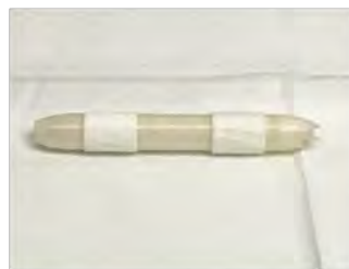
Cylindrical PSIS scaffolds mounted on sample holder of Torpedo Bioreactor
