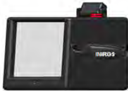
Integrated near-infrared optical scanner (I-NIROS) for oxygenation measurements
